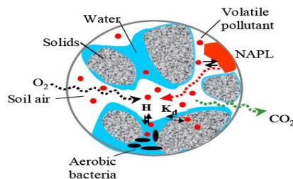
Figure 2: Conceptual model for a VOC biodegradation in unsaturated porous media
