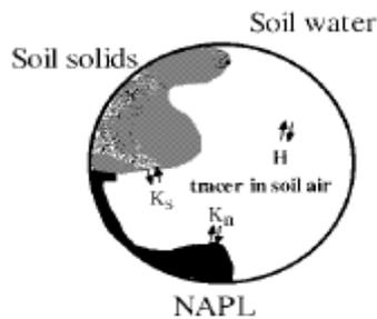
Figure 1. Equilibrium consideration for the soil gas tracers in an NAPL-contaminated soil [23].
